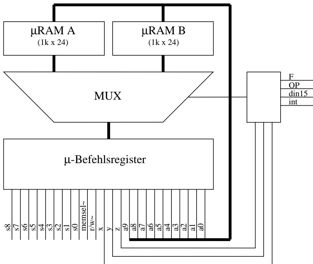
The three bits  $x, y, z$  determine, whether microword A or B is stored into the micro instruction register:
